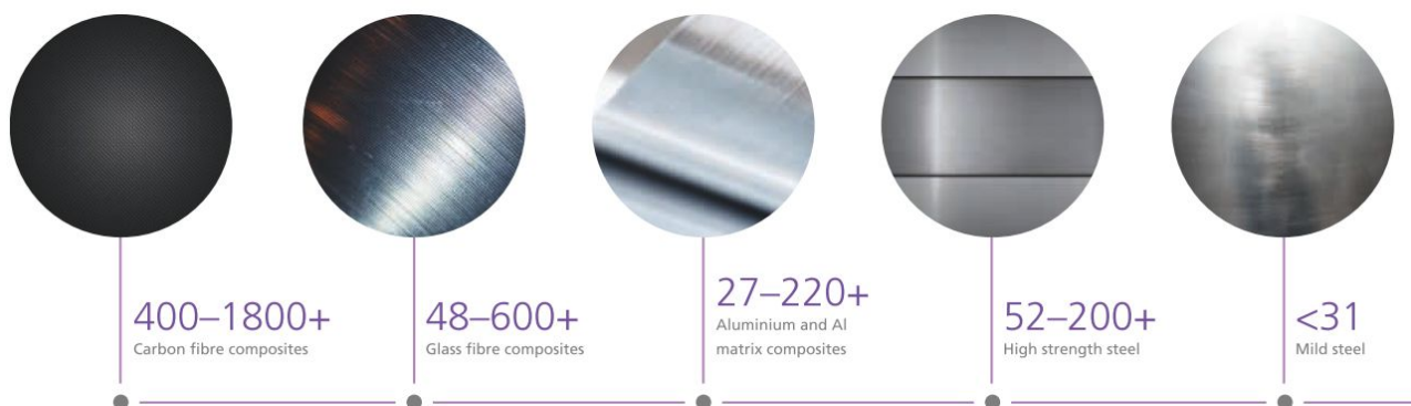
Figure 1: Strength-to-weight ratio of selected materials (kN*m/kg) [Lloyd's, 2015]
