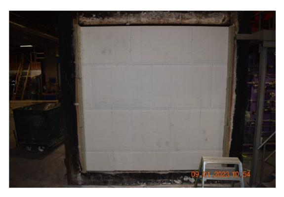
Photo No. 9 Gypsum mounted on exposed side of specimen.
