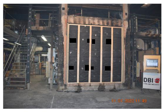
Photo No. 15 Unexposed side after 90 minutes of testing. Liquid is starting to run down the bottom of the specimen.
