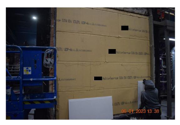
Photo No. 7 Mounting of gypsum boards, exposed side.
