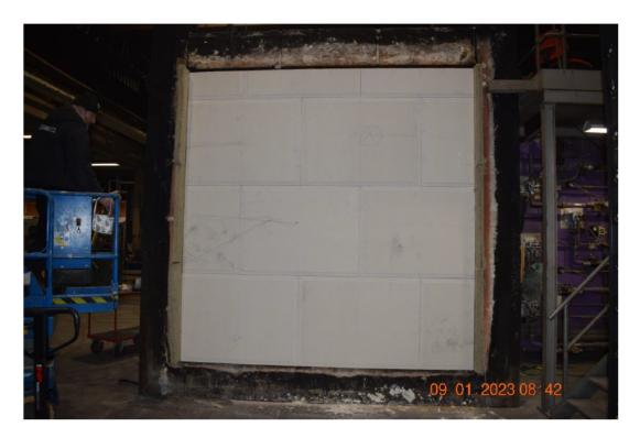
Photo No. 8 Gypsum mounted on exposed side of specimen.
