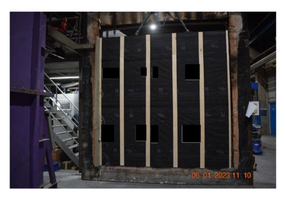
Photo No. 5 Unexposed side finished with wood spacers.
