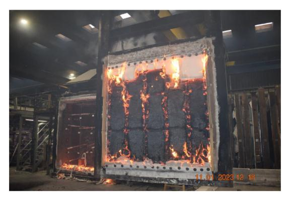
Photo No. 21 Unexposed side after test ended.
