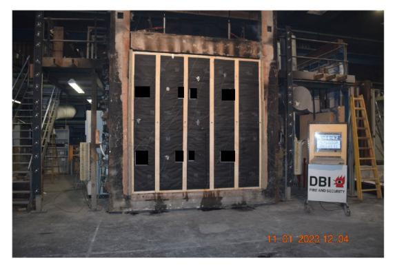
Photo No. 16 Specimen after 104 minutes of testing.
