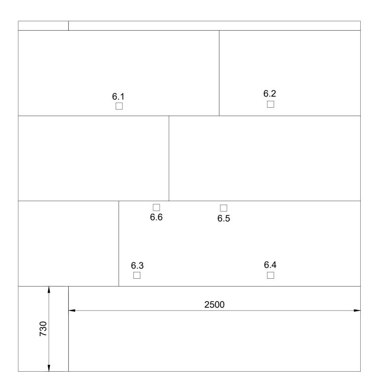
The wood fiber boards with tongue and groove have maximum dimensions of 750 x 2500 mm.
