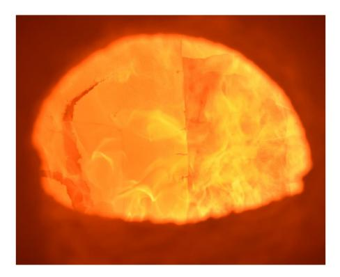
Photo No. 14 Exposed side of specimen after 90 minutes of testing.
