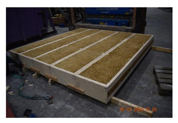
Photo No. 3 Wall element assembly finished.
