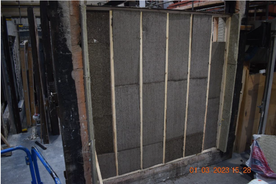
Photo No. 2 Timber frame of specimen, with seaweed insulation.
