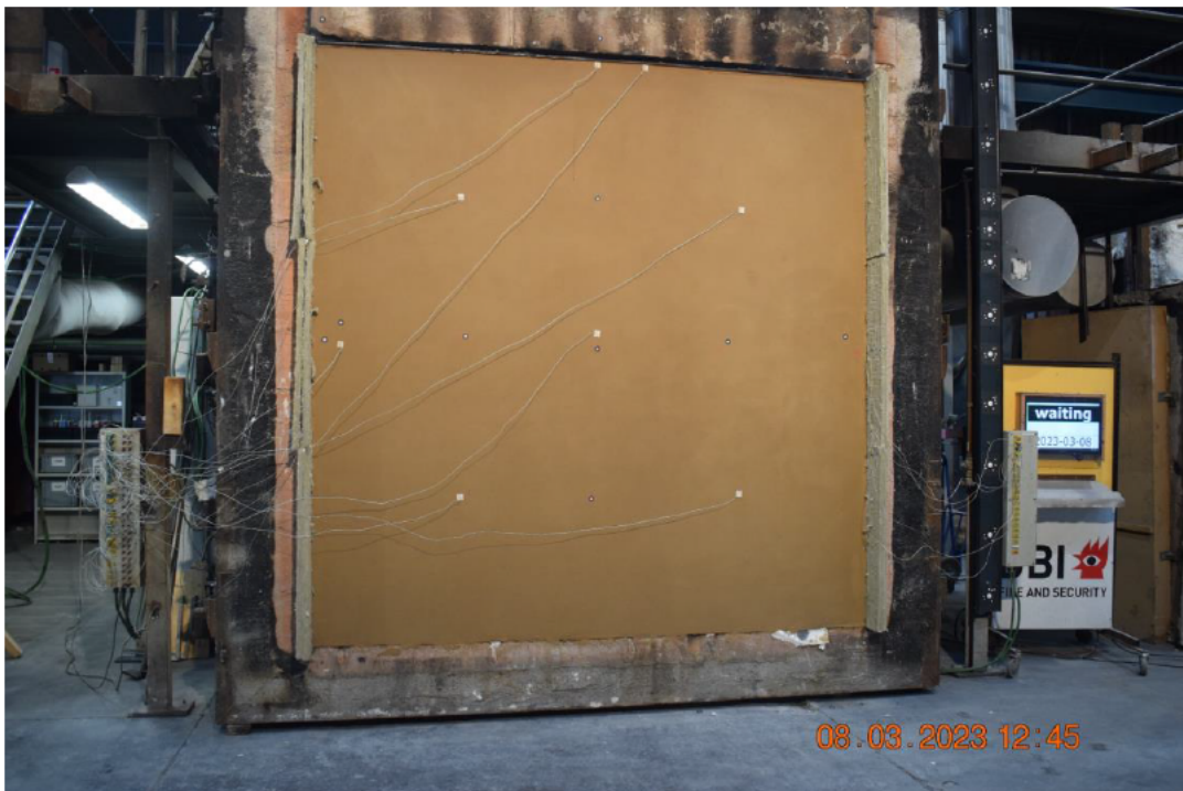
Photo No. 9 Test specimen seen from unexposed side after 42 minutes of testing
