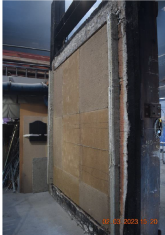
Photo No. 5a Test specimen seen from exposed side – inner layer of clay boards.
