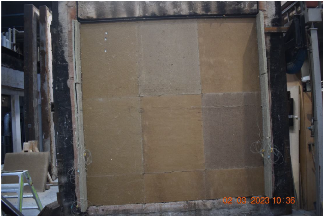
Photo No. 4a Unexposed side of test specimen, inner layer of clay boards.
