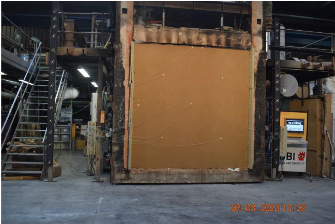
Photo No. 10 Test specimen seen from unexposed side after 60 minutes of testing
