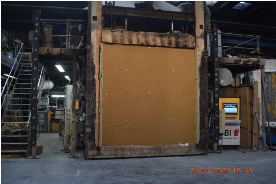
Photo No. 8 Test specimen seen from unexposed side after 30 minutes of testing
