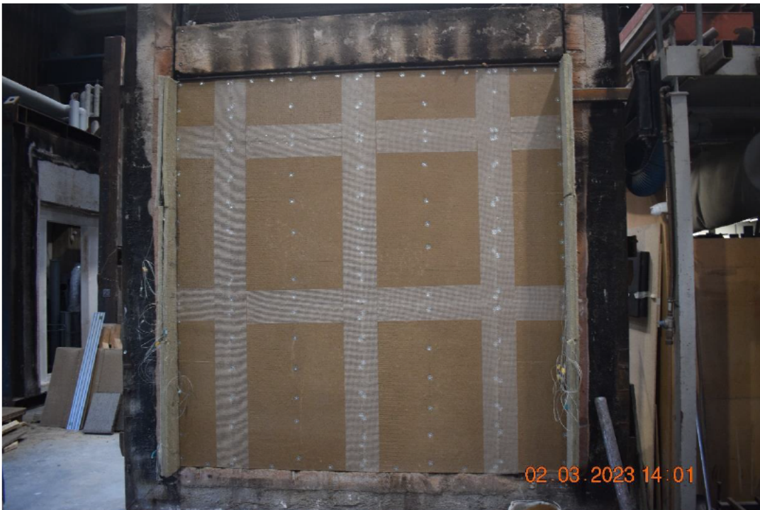
Photo No. 4b Unexposed side of test specimen, outer layer of clay boards, before clay plaster was added.
