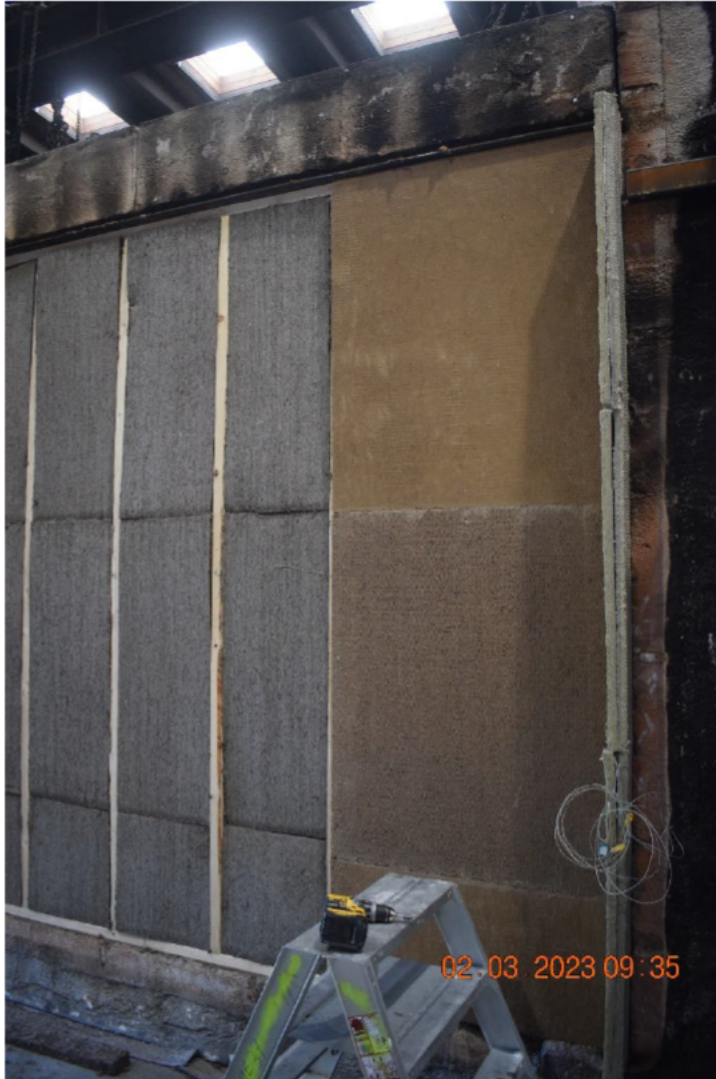
Photo No. 3 Timber frame of specimen, with seaweed insulation and first layer of clay board
