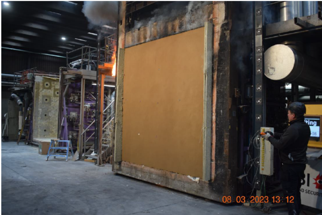
Photo No. 12 Test specimen after test seen from unexposed side
