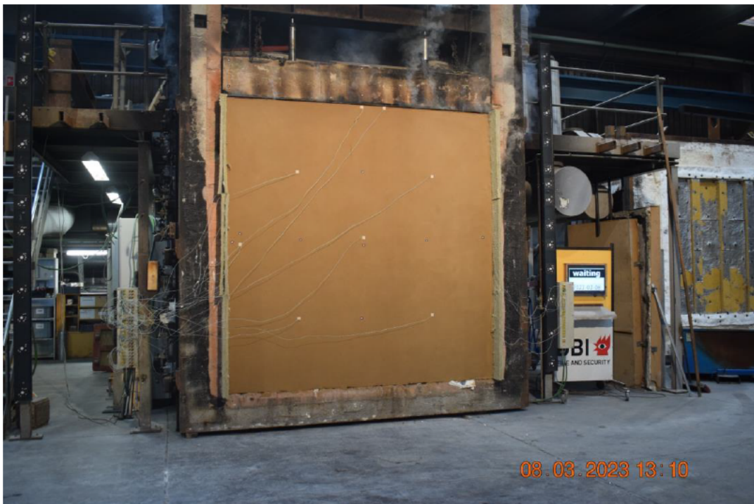
Photo No. 11 Test specimen seen from unexposed side after 67 minutes of testing
