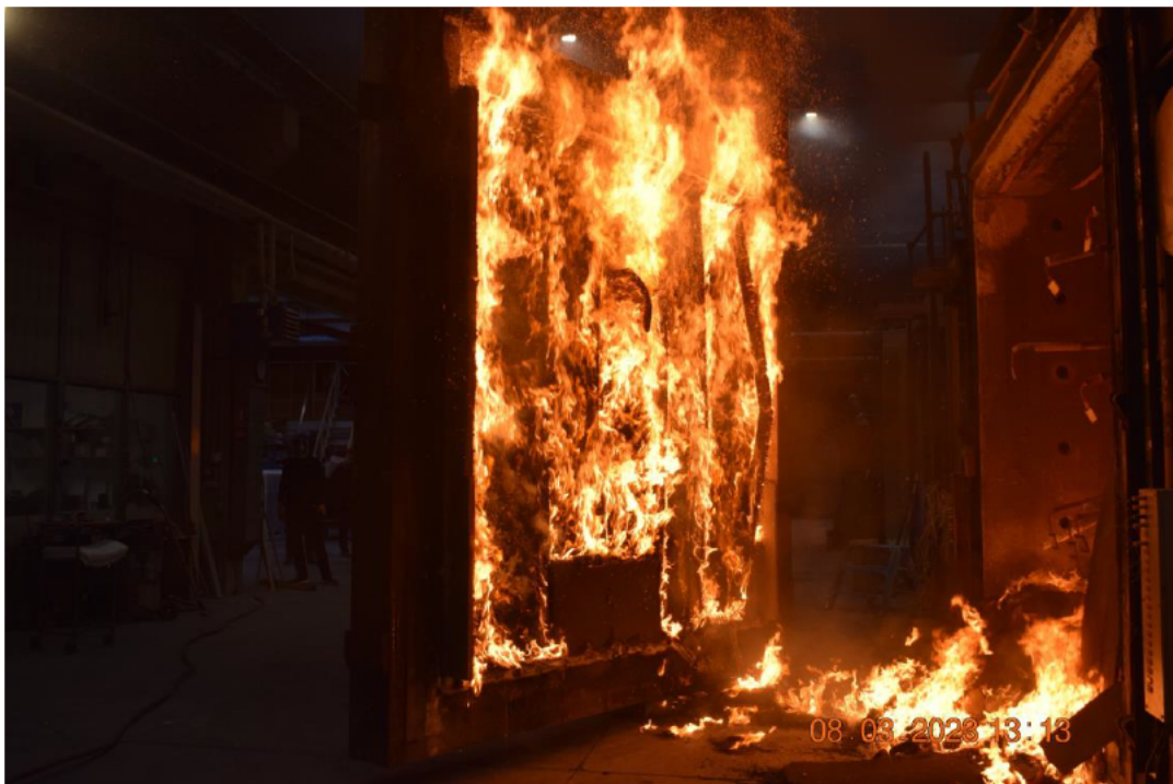
Photo No. 13 Test specimen seen from exposed side right after test
