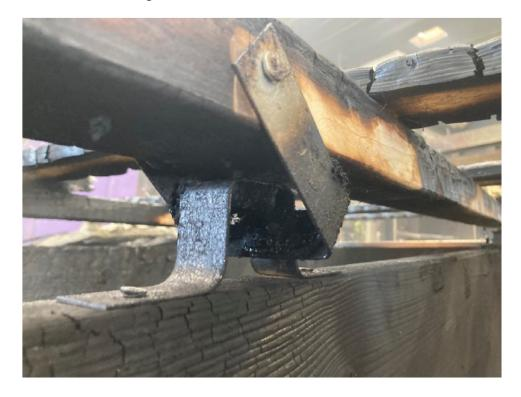
Photo No. 29 The sound dampening device after the test
