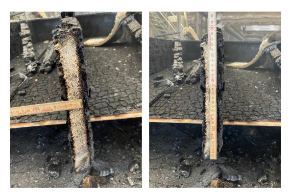
Photo No. 28 The loadbearing beams after the test
