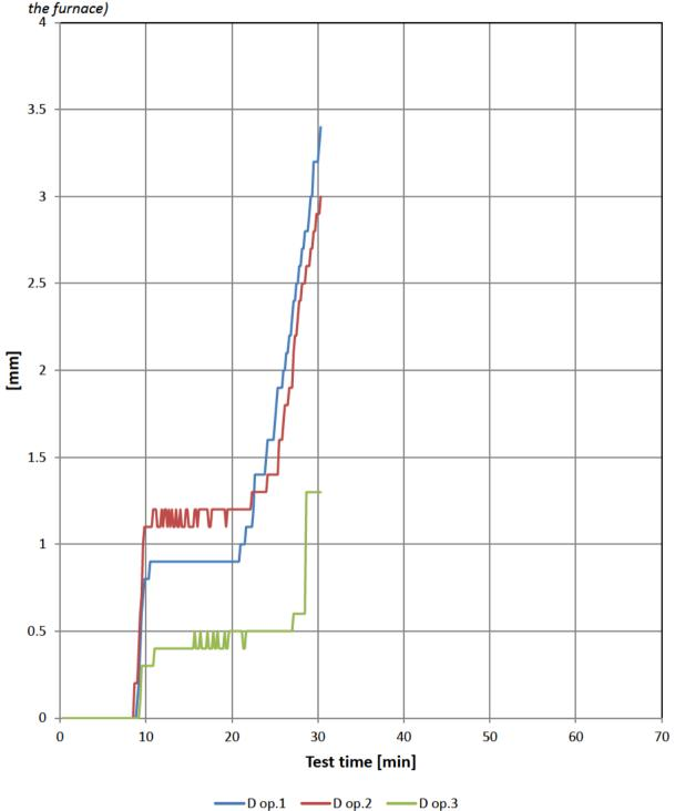
The vertical deflection measured on the unexposed side (positive values indicates movment towards the furnace)
