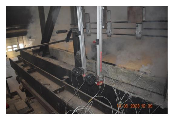
Photo No. 24 Test specimen seen from unexposed side at 60 minutes into testing
