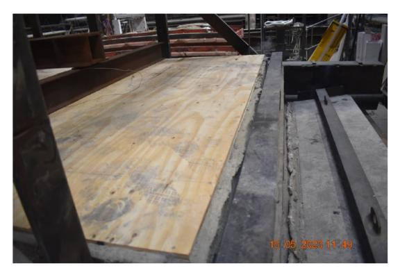
Photo No. 18 Test specimen seen from unexposed side 10 minutes into testing
